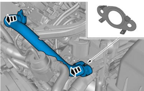
**Note!** Make sure that the seal is correctly located.
